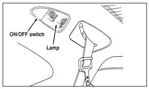
*Rear seat courtesy/reading lamps*
